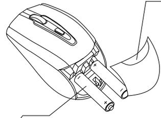
Correctly installing batteries according to the instruction
