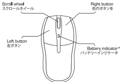
\*Battery indicator will blink frequency during the low voltage level
